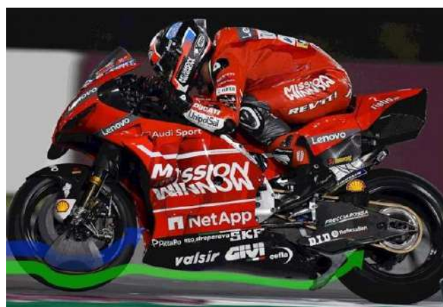
Figure 9: Ducati GP19 ground effect (Picture courtesy of: Sky Sport)
