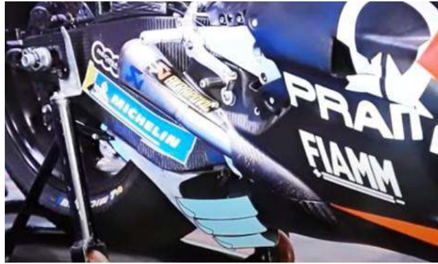
Figure 3: Ducati GP19 Swingarm Attachment device, 3 split elements
