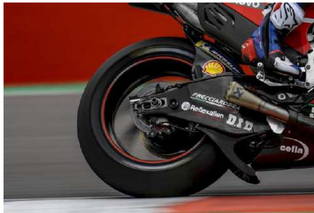
Figure 2: Ducati GP19 Swingarm Attachment device (Picture courtesy of: https://www.corsedimoto.com/motomondiale/motogp/motogp-la-tecnica-lo-spoiler-ducatti-quante-polemiche/ )
